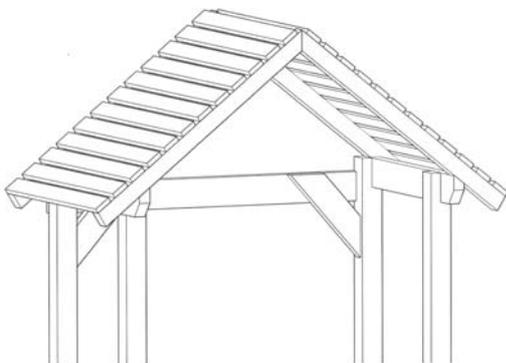
Lift the assembled roof sections into position. The roof should be flush with the back of the arbour. Secure the roof in place using 1 x 70mm screw placed through each corner into the posts of the arbour.
